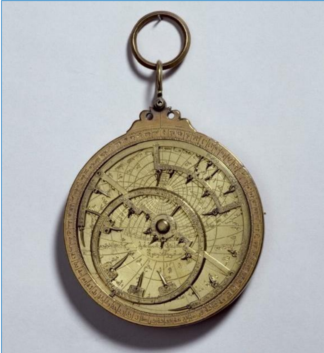
Figure 1 Astrolabe (Saragossa, 1079/80) featuring both Arabic and Latin writing. The circles of altitude parallel to the horizon are called almucantarats . They relate to a certain latitude. On the astrolabe, these circles are rendered as engravings around the zenith (in the upper half of the disc reproduced above). © Nuremberg, Germanic National Museum, Kat. 155.
