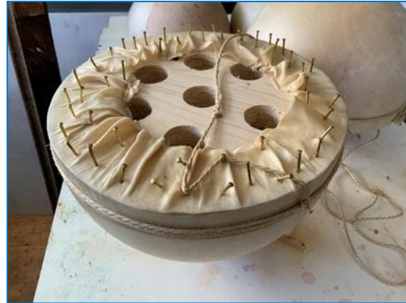
Figure 14 Covering of the calottes with parchment using a special clamping device. Photo: Hanspeter Strang.
